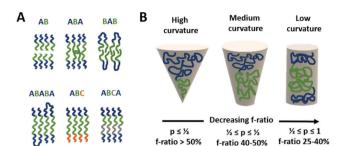
Fig. 2 (A) Schematic representation of different membrane architectures resulting from different copolymer structures. (B) Influence of the copolymer's f-ratio on the membrane curvature and the morphology of the self-assembly
