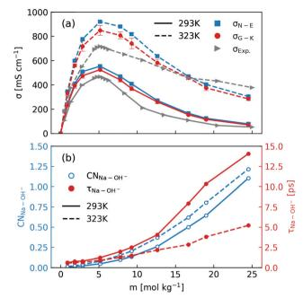
Fig. 1 (a) Comparison of concentration-dependent ionic conductivities calculated using the Nernst-Einstein formula (eqn (1) and (3)) and the Green-Kubo formula (egn (5)) from MD simulations and those measured in experiments at 293 K and 323 K; (b) calculated Na<sup>+</sup>-OH<sup>-</sup> coordination numbers and residence time
