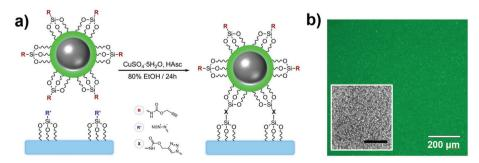
Fig. 10 (a) Grafting scheme of Ag@(FL) NPs to a SiO<sub>2</sub> substrate through Cu<sup>1</sup>-catalyzed 1,3-dipolar cycloaddition. (b) Fluorescence image of the substrate grafted with Ag@(FL) NPs ( $\lambda_{exc} = 489 \pm 6$  nm,  $\lambda_{em} = 536 \pm 20$  nm). Inset: SEM image of a region the substrate (scale bar: 1 µm). Adapted from ref. 115 with permission from the Royal Society of Chemistry, Copyright 2014.
