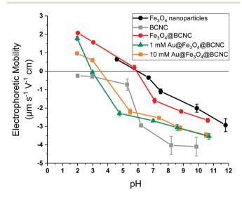
Fig. 3 Electrophoretic mobility of bare Fe<sub>3</sub>O<sub>4</sub> nanoparticles, BCNCs, Fe<sub>3</sub>O<sub>4</sub>@BCNCs, 1 mM and 10 mM Au@Fe<sub>3</sub>O<sub>4</sub>@BCNCs in 0.01 M NaCl solution. The error bars indicate standard deviation of three measurements.
