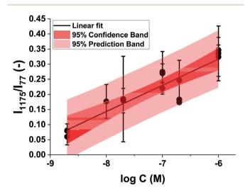
Fig. 6 The comprehensive plot of the normalized Raman peak of 1175 cm<sup>-1</sup> vs. the logarithm of the concentrations of MGITC using 1, 5, and 10 mM Au@Fe<sub>3</sub>O<sub>4</sub>@BCNCs. The black solid line shows the best-fit linear curve. Dark and light red-colored regions show statistical 95% confidence and prediction bands, respectively.  $R^2 = 0.79$ , Linear fit:  $I_{1175}/I_{1175}$  $I_{77} = 0.837 + 0.087 \log C$ .
