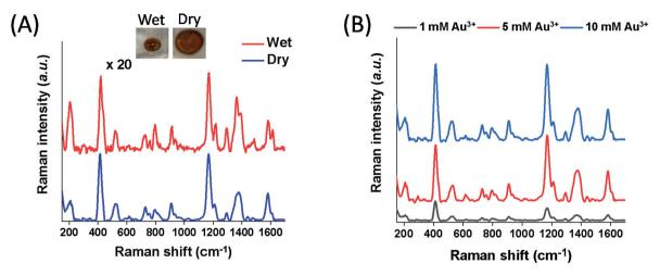
Fig. 4 (A) Comparison of the SERS spectra of 2  $\mu$ M MGITC under wet and dry conditions using 10 mM Au@Fe<sub>3</sub>O<sub>4</sub>@BCNCs. Inset pictures show before/after drying of 10  $\mu$ L of the droplet including the nanocomposites. (B) The SERS spectra of 2  $\mu$ M MGITC using the Au@Fe<sub>3</sub>O<sub>4</sub>@BCNCs with different Au coating condition (1, 5, and 10 mM Au<sup>3+</sup>). All spectra shown here are the average of 400 collected spectra.
