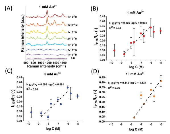
Fig. 5 SERS detection of MGITC using the Au@Fe $_3O_4$ @BCNCs. (A) The SERS spectra of MGITC with the different concentrations using 1 mM Au@Fe $_3O_4$ @BCNC stacked vertically for clarity. (B)–(D) The plots of the normalized peak of 1175 cm $^{-1}$  ( $I_{1175}/I_{77}$ ) vs. the logarithm of concentrations of MGITC using 1, 5, and 10 mM Au@Fe $_3O_4$ @BCNCs. Symbol and error bar represent the average and standard deviation of 400 spectra for each point, respectively.
