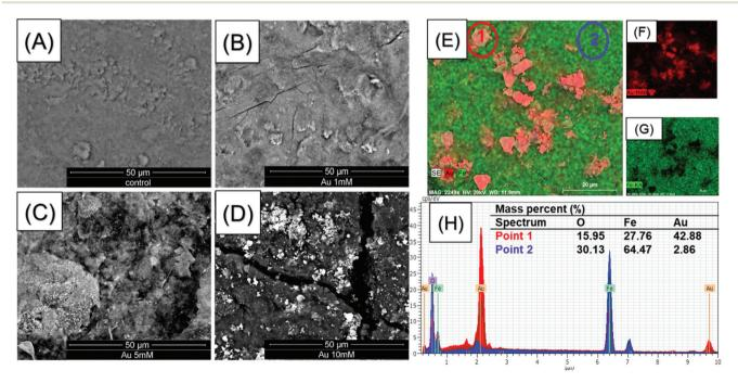
Fig. 2 Backscattered SEM images of the aggregated (A) Fe<sub>3</sub>O<sub>4</sub>@BCNCs, (B) 1 mM Au@Fe<sub>3</sub>O<sub>4</sub>@BCNCs, (C) 5 mM Au@Fe<sub>3</sub>O<sub>4</sub>@BCNCs and (D) 10 mM Au@Fe<sub>3</sub>O<sub>4</sub>@BCNCs. EDS mapping of (E) 10 mM Au@Fe<sub>3</sub>O<sub>4</sub>@BCNCs with (F) Au and (G) Fe elements highlighted. The corresponding (H) EDS spectra of the map are provided with mass percent of O, Fe, and Au shown.
