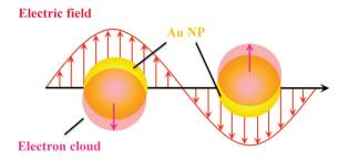
Fig. 1 Schematic illustration of the origin of LSPR.
