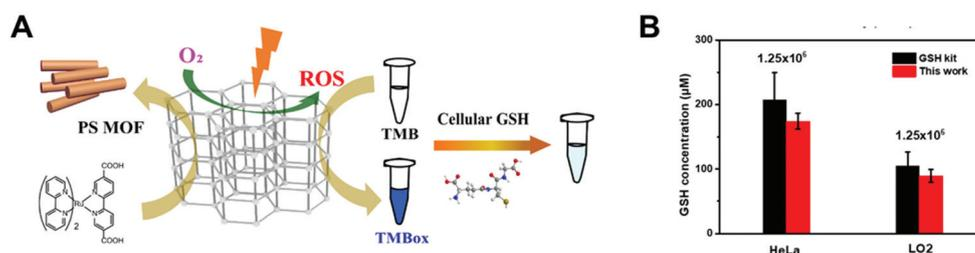
**Fig. 9** (A) Schematic illustration of the cellular GSH detection by using a PS MOF-based photoactive sensor. (B) Qualitative evaluation of cellular GSH levels with the developed sensor and a GSH kit. The number marked on the histogram is the cell density. Each error bar shows the standard deviation of three independent measurements. Reproduced from ref. 84 with permission from the American Chemical Society, copyright 2019.
