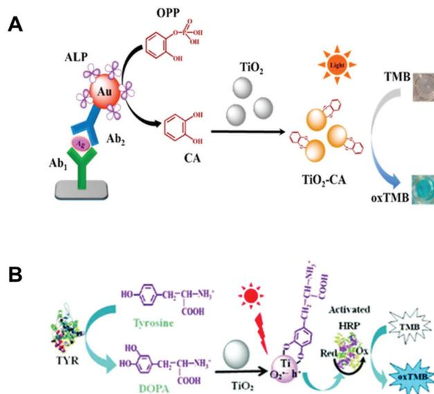
Fig. 7 (A) Proposed immunodetection process for mouse IgG by coupling the *in situ*-generated photo-responsive nanozyme of CA-TiO<sub>2</sub>. (B) Schematic illustration of the colorimetric sensing mechanism for TYR based on the photoactive sensor. (A) Reproduced from ref. 79 with permission from the American Chemical Society, copyright 2015. (B) Reproduced from ref. 80 with permission from the Royal Society of Chemistry, copyright 2017.
