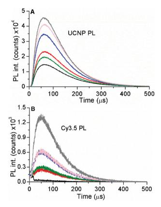
Fig. 3 Time-resolved PL intensities of c-UCNPs (A,  $\lambda_{\rm em}=542\pm10$  nm) and Cy3.5 (B,  $\lambda_{\rm em}=607\pm5$  nm) for different ratios of Cy3.5-ssDNA per c-UCNP (0.09 nmol mg $^{-1}$  – black; 0.47 nmol mg $^{-1}$  – red; 0.97 nmol mg $^{-1}$  – green; 1.89 nmol mg $^{-1}$  – blue; 2.46 nmol mg $^{-1}$  – pink; 3.54 nmol mg $^{-1}$  – gray) in water upon excitation at 980 nm. The concentration of c-UCNPs was constant (1 mg mL $^{-1}$ ).
