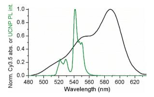
Fig. 2 The green PL bands of UCNPs (green) overlap with the absorption spectrum of Cy3.5 (black). See ESI $\dagger$  for calculation of overlap integrals.
