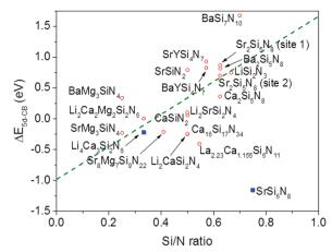
Fig. 7  $\Delta E_{\rm 5d-CB}$  versus the Si/N ratio in the Eu<sup>2+</sup> doped nitridosilicates. The straight line is a linear fit through the red data points. The blue squared data points represent exceptions discussed in the text.
