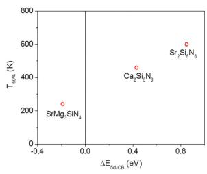
Fig. 5 Temperature at which 50% of the Eu<sup>2+</sup> 5d-4f emission is quenched  $(T_{50\%})$  versus the energy difference ( $\Delta E_{\rm 5d-CB}$ ) between the bottom of the host lattice conduction band and the lowest relaxed Eu<sup>2+</sup> 5d state for SrMg<sub>3</sub>SiN<sub>4</sub>:Eu<sup>2+</sup>, Ca<sub>2</sub>Si<sub>5</sub>N<sub>8</sub>:Eu<sup>2+</sup> and Sr<sub>2</sub>Si<sub>5</sub>N<sub>8</sub>:Eu<sup>2+</sup>.
