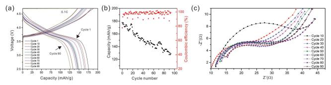
Fig. 6 (a) The cycling curves, (b) capacity and coulombic efficiency, and (c) impedance curves of the hybrid cell from the 1st to the 90th cycle.
