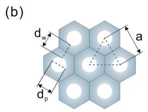
Fig. 8 (a) The 3D model and (b) top view of the simplified honeycomb structure of the porous LLZO scaffold.
