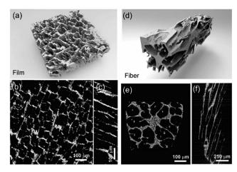
Fig. 3 The 3D reconstructed structure from the SR- $\mu$ CT data of (a) the LLZO film and (d) longitudinal section. The cross-sections for the film are shown in (b) top and (c) left views. (e) and (f) are the top and left views of the LLZO longitudinal section.
