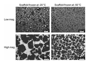
Fig. 4 SEM top views of the sintered LLZO scaffolds, frozen at -20 °C and -50 °C, respectively, at low and high magnifications.
