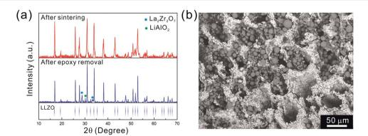
Fig. 5 (a) XRD pattern of the scaffold after sintering and after epoxy removal, respectively. The LLZO XRD peaks are indicated in the lower part. (b) SEM image of the scaffold flipped over after drop casting of NMC particles from the other side.
