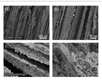
Fig. 2 SEM images of the fractured LLZO scaffolds (a and b) before and (c and d) after sintering.
