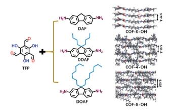
Fig. 2 The formation of COF-0-OH, COF-4-OH, and COF-8-OH to reveal the effects of alkyl groups on the interlayer spacings of different COFs.
