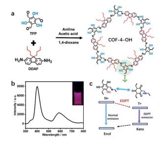
Scheme 1 (a) The design of COFs to reveal the effects of hydroxyl and alkyl groups and the ESIPT procedure, showing hydroxyl-functional TFP and alkyl groups-containing DDAF for the preparation of COF-4-OH. (b) Dual emission from COF-4-OH under 280 nm excitation; inset: a picture of COF-4-OH under 280 nm illumination. (c) The ESIPT dual emission mechanism of hydroxyl-containing COF-4-OH.
