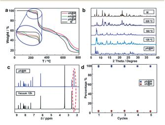
Fig. 4 Recyclability of M. (a) The TGA profiles for M, oX@M, mX@M, pX@M. Loss of weight: pX@M > mX@M > oX@M. (b) VT-XRD experiments for pX@M. With the temperature increasing, the pattern of PXRD transformed from pX@M into M. (c) The <sup>1</sup>H NMR spectra of pX@M and the sample after vacuum drying. (d) Relative uptake of pX and oX in Mafter M is recycled for 5 times
