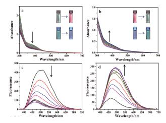
Fig. 4 Absorption spectral changes of Eu³+ $\subset$  $\gamma$ -CD· $\mathbf{1}_2$  (0.1 mM) upon irradiation (a) at 365 nm and (b) at 254 nm in PBS at 25 °C (pH = 7.2, inset: the upper and lower images for the fluorescence changes at an excitation wavelength of 254 nm and 365 nm, respectively). Fluorescence spectral changes of Eu³+ $\subset$  $\gamma$ -CD· $\mathbf{1}_2$  upon photoirradiation (c) at 365 nm and (d) at 254 nm in PBS at 25 °C ( $\lambda_{ex}$  = 365 nm).
