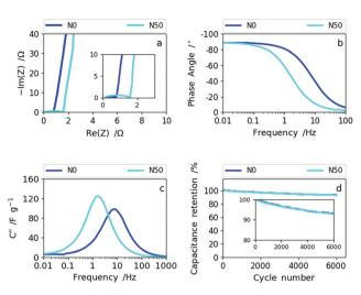
Fig. 7 (a) The Nyquist plots of NO and N50, (b) Bode phase angle plots of N0 and N50, (c) imaginary capacitance vs. frequency dependencies of N0 and N50 and (d) cyclability data of N0 and N50.
