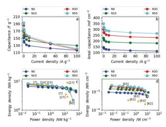
Fig. 8 (a) Dependence of specific gravimetric capacitance on current density for all four samples; (b) dependence of specific areal capacitance on current density for all four samples; (c) Ragone plot in gravimetric measures and (d) Ragone plot in volumetric measures.
