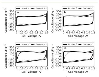
Fig. 6 Voltammograms at 10 and 500 mV s $^{-1}$  of (a) N0, (b) N10, (c) N30, and (d) N50 measured in 6 M KOH.
