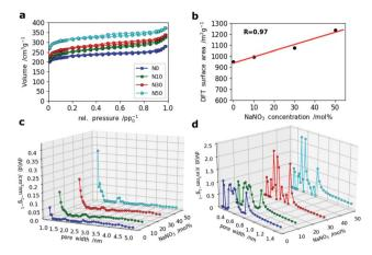
Fig. 5 (a)  $N_2$  sorption isotherms of all four samples, (b) correlation of DFT-derived surface area and  $NaNO_3$  content, (c) PSDs calculated by DFT (QSDFT (slit pore/cylindrical pore) model) based on the adsorption isotherms of  $N_2$  and (d) PSDs from  $CO_2$  adsorption measurements (NLDFT, Non-Localized DFT method).
