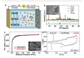
Fig. 1 (a) Schematic illustration of the KIHC with the configuration K<sub>2</sub>TP//DME-based electrolyte//AC; (b) XRD pattern, Rietveld-refined profile, and SEM image (inset) of K<sub>2</sub>TP; (c) nitrogen sorption isotherm and SEM image (inset) of AC; and (d) CV curves of half batteries and the KIHC
