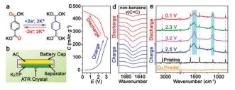
Fig. 2 (a) Redox reaction mechanism of  $K^+$  with  $K_2TP$ ; (b) diagram of a cell for *in situ* FTIR test; (c) charge/discharge profile of the KIHC at 20 mA  $g^{-1}$  (based on the mass of  $K_2TP$ ); (d) *in situ* FTIR spectra of the  $K_2TP$  negative electrode in a charge/discharge cycle; and (e) Raman spectra of the  $K_2TP$  negative electrode at selected states with copper powder.
