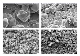
Fig. 2 SEM images of polyUiO-66 prepared from block copolymer ligands: (a) pbdc-8a-PE $G_{2000}$ -2%; (b) pbdc-8a-PE $G_{4000}$ -1%; (c) pbdc-8a-PE $G_{2000}$ -20%; (d) pbdc-8a-PE $G_{4000}$ -10%.
