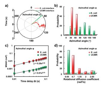
Fig. 5 (a) The angular rotational trajectories of E. coli and UCMRs on the lipid membrane in the x-y plane. (b) The azimuthal angle distributions of E. coli and UCMRs. (c) Representative MSAD plots of E. coli and UCMRs from the azimuthal angle on the lipid membrane. (d) The distribution of the rotational diffusion coefficients of E. coli and UCMRs on the lipid membrane in the x-y plane.
