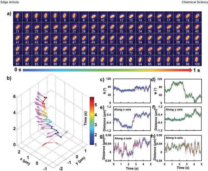
(a) Frame-by-frame images of the rotational and translational diffusion of E. coli on the lipid membrane with an observation time window of 1 s. (b) The time-dependent trajectory of E. coli on the lipid membrane. The 3D orientations from different time periods are marked with red arrows. (c)–(h) The time-dependent trajectories from the polar angle, the azimuthal angle, the walking displacement along x and y axes, and the walking displacement along a and b axes, respectively.
