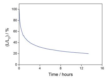
Fig. 10 Relative luminance of vacuum-deposited OLEDs based on 5 wt% complex 7 as a function of operation time at a constant driving current density of 20 mA cm $^{-2}$ .
