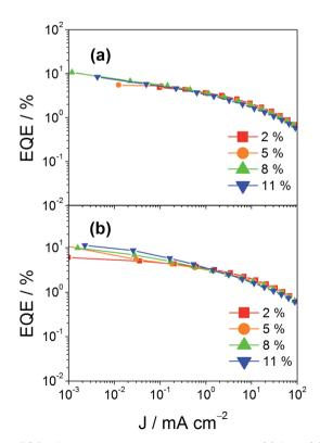
Fig. 9 EQEs of vacuum-deposited devices made with (a) 4 and (b) 7 at different concentrations.
