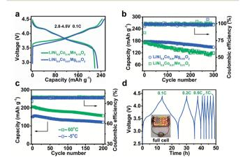
Fig. 3 (a) Initial charge and discharge curves at 0.1C rate and (b) cycling performance of LiNi $_{0.9}$ Co $_{0.07}$ Mg $_{0.03}$ O $_2$  and NCM811 at 2C rate for 300 cycles. (c) LiNi $_{0.9}$ Co $_{0.07}$ Mg $_{0.03}$ O $_2$  performance at a temperature of -5 and 60 °C at 1C. (d) Charge/discharge profiles of the full LIB cell assembled with the LiNi $_{0.9}$ Co $_{0.07}$ Mg $_{0.03}$ O $_2$  cathode and graphite anode. The inset shows a cell powering a string of LIB-shaped LED lights.
