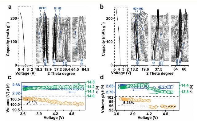
Fig. 4 Structural evolution of LiNi<sub>0.9</sub>Co<sub>0.07</sub>Mg<sub>0.03</sub>O<sub>2</sub> (a and c) and NCM811 (b and d). (a and b) In situ XRD patterns at selected  $2\theta$  regions and the corresponding galvanostatic curves on first charging. (c and d) The variation of lattice parameters and cell volumes as a function of voltage.
