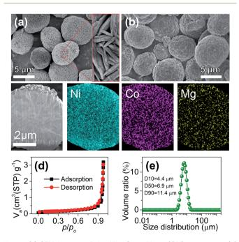
Fig. 1 (a) SEM images of the Ni<sub>0.9</sub>Co<sub>0.07</sub>Mg<sub>0.03</sub>(OH)<sub>2</sub> precursor. (b) SEM image, (c) cross-sectional elemental mapping, (d) N<sub>2</sub> adsorption/ desorption isotherms and (e) particle size distribution of the synthesized LiNi $_{0.9}$ Co $_{0.07}$ Mg $_{0.03}$ O $_{2.03}$
