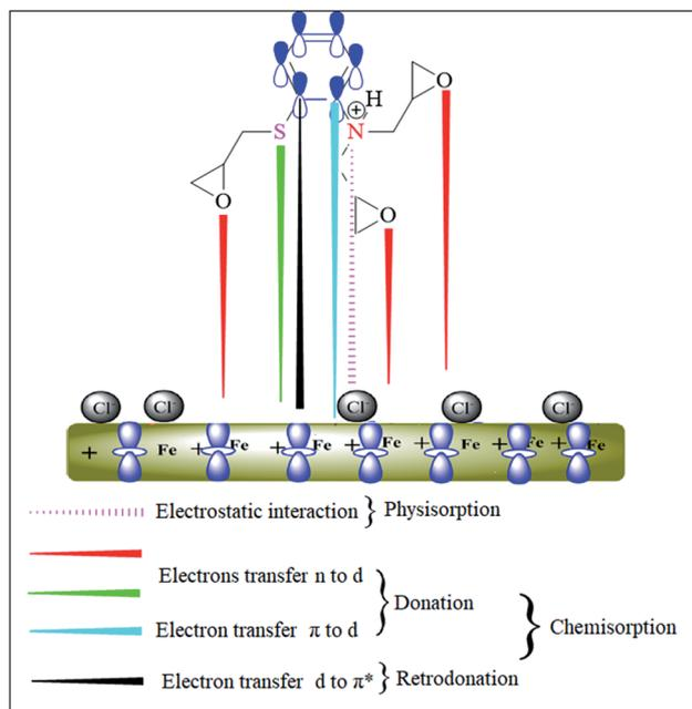
Fig. 11 Pictorial representation of adsorption of AEM2 on carbon steel surface in 1 M HCl solution.
