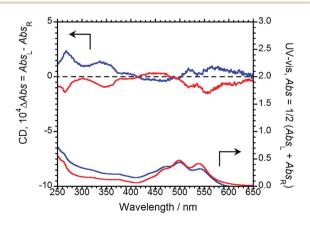
Fig. 5 CD (upper) and UV-Vis (lower) absorption spectra of (R,R)-BPP (blue) and (S,S)-BPP (red) in KBr-pellet-dispersed states.
