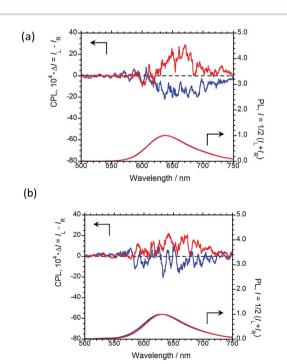
Fig. 6 CPL (upper) and PL (lower) spectra of (R,R)-BPP (blue) and (S,S)-BPP (red) in (a) PMMA-film- and (b) myo-IPU-film-dispersed states.
