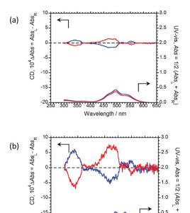
Fig. 7 CD (upper) and UV-Vis absorption (lower) spectra of (R,R)-BPP (blue) and (S,S)-BPP (red) in (a) PMMA-film- and (b) myo-IPU-film-dispersed states.
