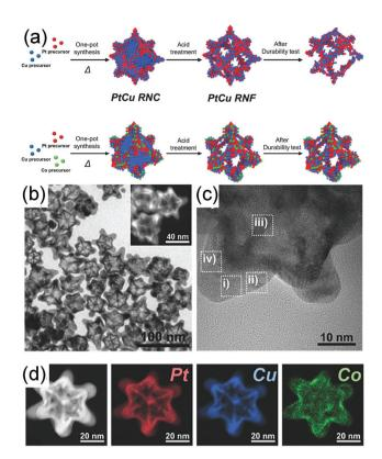
Fig. 11 (a) Schematic illustration of the formation process of PtCu RNC, PtCu RNF, Co-PtCu RNC, and Co-PtCu RNF. (b)TEM and (c) HRTEM images and (d) HAADF-STEM image and corresponding EDS elemental mapping analysis of Co-PtCu RNF. Adapted with permission from ref. 24. Copyright 2018, Wiley-VCH.
