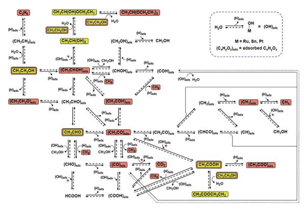
Fig. 17 Ethanol electrochemical reaction pathways on Pt-based catalysts. The reaction steps marked with red stars are those in which (OH)<sub>ads</sub> are involved and catalytic sites are regenerated due to reaction with (OH)<sub>ads</sub>. The chemical species highlighted in yellow were observed in this study, and those highlighted in brown were observed in earlier studies that used other analytical techniques. Adapted with permission from ref. 194. Copyright 2011, Wiley-VCH.
