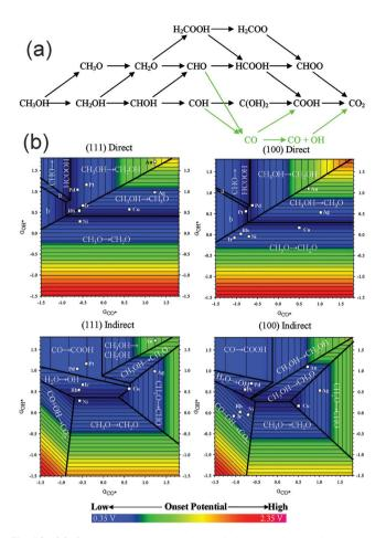
Fig. 16 (a) Schematic representation of the reaction pathways and possible intermediates considered here for methanol electrooxidation. Green arrows indicate the indirect mechanism to CO<sub>2</sub> formation. (b) Potential-determining steps for methanol electrooxidation on (111) and (100) facets plotted using  $G_{CO^*}$  and  $G_{OH^*}$  as the descriptors. Adapted with permission from ref. 190. Copyright 2009, American Chemical Society.
