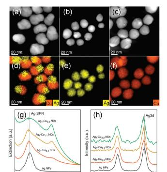
Fig. 25 (a-c) HAADF-STEM images of Aq1-Cu1.1 NDs (a), Aq NPs (b), and Cu NPs (c); (d-f) corresponding EDX elemental maps of Cu (orange) and Ag (yellow) of Ag1-Cu1.1 NDs (d), Ag NPs (e), and Cu NPs (f). (g) UV-vis spectra and (h) XPS spectra of Ag/Cu nanocrystals. Adapted with permission from ref. 279. Copyright 2019, American Chemical Society.
