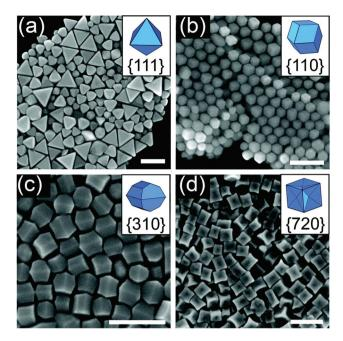
Fig. 6 SEM images of (a) octahedra, (b) rhombic dodecahedra, (c) truncated ditetragonal prisms, and (d) concave cubes of Au–Ag synthesized from reaction solutions containing  $Ag^+/Au^{3+}$  ratios of 1:500, 1:50, 1:12.5, and 1:5, respectively. Scale bars: 200 nm. Adapted with permission from ref. 86. Copyright 2018, American Chemical Society.
