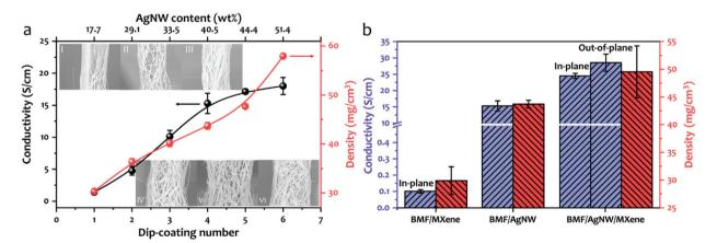
Fig. 3 (a) Conductivity and mass density of the BMF/AgNW sponge at different dip-coating cycles. Insets are SEM images of AgNW coated backbone of the BMF sponge. (b) The comparison of conductivity and mass density of BMF/MXene, BMF/AgNW and BMF/AgNW/MXene sponges.
