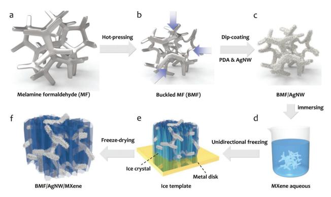
Fig. 1 Schematic illustrating the fabrication process of the BMF/AgNW/MXene hybrid sponge by a combination of mechanical hot-pressing ( $a\rightarrow b$ ), dip-coating ( $b\rightarrow c$ ), immersing ( $c\rightarrow d$ ), unidirectional freezing ( $d\rightarrow e$ ), and freeze-drying ( $e\rightarrow f$ ).
