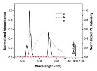
Fig. 2 UCL spectrum of DSPC-coated NaYF<sub>4</sub>:20%Yb,2%Er (DSPC-UCNPs) under excitation from a 980 nm laser (a), and UV-vis spectra of the protein apo-azurin in the absence (b) and presence of  $Cu^{2+}$  (c).
