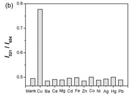
Fig. 6 (a) Changes in the absorption spectra of apo-azurin upon addition of one eq. of various metal ions; (b) the ratio ( $I_{521}/I_{654}$ ) of UCL intensities at 521 and 654 nm of the sensor system (under excitation from a 980 nm laser) in the presence of various representative metal ions (64  $\mu$ M Cu<sup>2+</sup> and 100  $\mu$ M other metal ions).
