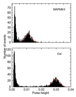
Fig. 4 Pulse height spectra of scintillations excited through  $\alpha$ -particle interaction from <sup>241</sup>Am in MAPbBr<sub>3</sub> at 50 K and CsI at 50 K before correction for the spectral response of the photomultiplier. The pulse height distributions that signify scintillation response due to  $\alpha$ -particles are fitted by Gaussians (red lines).
