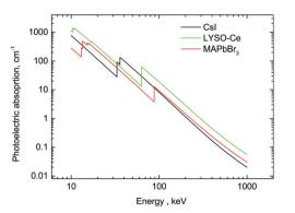
**Fig. 6** Photoelectric fractions of absorption of gamma-rays in Csl, LYSO-Ce and MAPbBr<sub>3</sub>. The data are calculated using an XCOM web-tool.<sup>50</sup>
