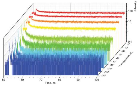
Fig. 1 X-ray data. Decay curves of X-ray luminescence measured in the MAPbBr<sub>3</sub> crystal at different temperatures in the range 8-132 K (where the emission is most pronounced). The luminescence is excited with 60 ps pulses of synchrotron radiation (E = 14 keV).
