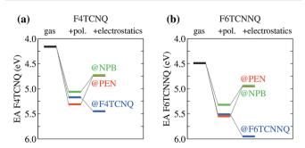
Fig. 3 EA of (a) F4TCNQ and (b) F6TCNNQ in different hosts dissected into its different contributions. Polarization and electrostatic terms are progressively added to gas-phase EA to highlight the origin of the pronounced host-dependence of energy levels arising from the latter effect. Notice the opposite electrostatic shifts for pure dopant crystals (e.g. F6TCNNQ@F6TCNNQ) and for dopants acting as impurities in a host OSC (e.g. F6TCNNQ@NPB)
