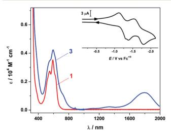
Fig. 2 Overlay of the electronic spectra of 1 and 3 recorded in CH<sub>2</sub>Cl<sub>2</sub> at ambient temperature. Inset shows the cyclic voltammogram recorded in 5:1 anisole/CH<sub>2</sub>Cl<sub>2</sub> containing 0.2 M [N(<sup>n</sup>Bu)<sub>4</sub>]PF<sub>6</sub> at 100 mV s<sup>-1</sup> with potentials referenced to the Fc<sup>+/0</sup> couple.
