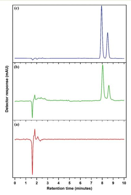
Fig. 6 Typical chromatogram obtained for the extraction of a water sample spiked with the two analytes under the optimum conditions: (a) non-spiked, (b) spiked with 100 ng  $mL^{-1}$  before DMSPE, and (c) extracted from a water sample after DMSPE of the analytes.
