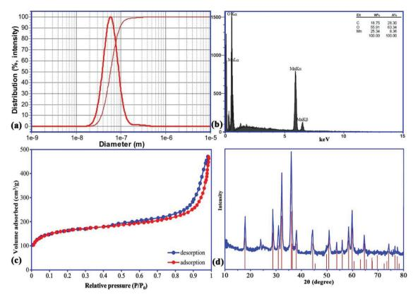
Fig. 2 Particle size distribution (a), EDX analysis (b), N<sub>2</sub> adsorption/desorption isotherms (c), and XRD pattern (d) of Mn<sub>3</sub>O<sub>4</sub>-NPs-AC.
