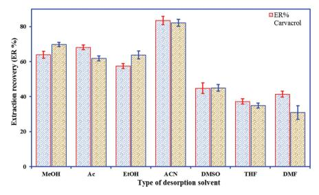
Fig. 3 Selection of the desorption solvent for the DMSPE experiments. Conditions: sample volume, 15.0 mL; desorption volume, 200  $\mu$ L; extraction time, 3 min; nano-sorbent mass, 10 mg; desorption time, 3 min; pH, 5.0; room temperature.
