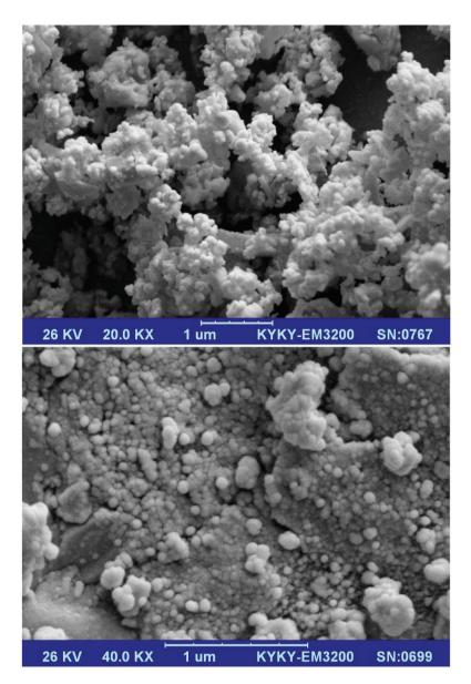
Fig. 1 SEM images of Mn<sub>3</sub>O<sub>4</sub>-NPs-AC at different magnifications.
