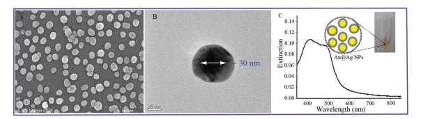
Fig. 3 (A) SEM image of Au@Ag NPs. (B) TEM image of Au@Ag NPs with a 30 nm Au core and a 7 nm Ag shell. (C) Extinction visible spectrum of Au@Ag NPs.
