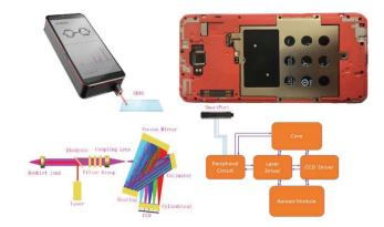
Fig. 1 The schematic illustration of the smartphone-based SERS analysis.
