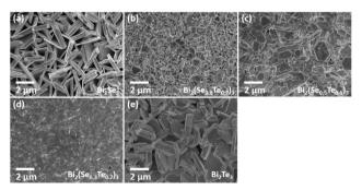
**Fig. 3** SEM images showing the morphologies of the  $Bi_2Se_3$  (a),  $Bi_2Te_3$  (e) and ternary  $Bi_2(Se_{1-x}Te_x)_3$  (b–d) films deposited by LPCVD under similar conditions (550 °C/0.05 mmHg) onto  $SiO_2$ -coated silicon substrates.
