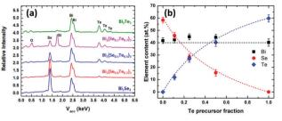
Fig. 2 (a) EDX spectra and (b) relationship between film composition and fraction of  $[BiCl_3(Te^nBu_2)_3]$  used in the deposition of ternary  $Bi_2(Se_{1-x}Te_x)_3$  films
