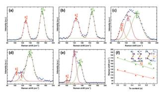
Fig. 5 (a–e) Raman spectra of as-deposited  ${\rm Bi_2(Se_{1-x}Te_x)_3}$  films with x ranging from 0 to 1. (f) Phonon frequencies (orange:  ${\rm E_g^2}$  mode; green:  ${\rm A_{1g}^2}$  mode) as a function of Te composition. The inset provides the schematic diagrams for the two Raman-active modes.
