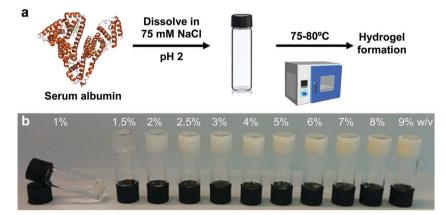
Fig. 1 Gelation of BSA solutions. (a) Protocol for hydrogel formation. (b) Image of the BSA hydrogels at different weight fractions ≥ 1.5 wt% BSA, together with a solution of 1 wt% BSA that did not gel after heating
