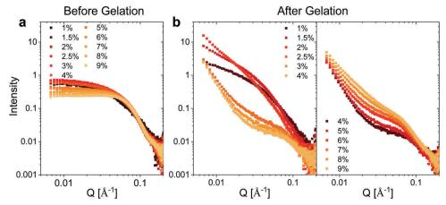
SAXS measurements. Concentration normalized SAXS intensity for the different weight fractions of BSA (a) before and (b) after gelation.
