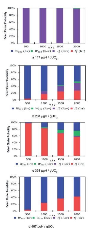
Fig. 5 Defect cluster probability at different local hydrogen concentrations as a function of temperature. The probability has been calculated relative to the most stable cluster for each local hydrogen concentration. Reversible  $W_{222}$  shown in green, irreversible  $W_{222}$  in blue, reversible  $V_{22}$  purple and irreversible  $V_{2}$  in red.
