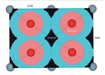
Fig. 2 Representation of hydrogen behavior in  $UO_2$  projected in a [110] direction. Black represents regions where hydride is predicted to be energetically most stable, light blue the H $^*$  radical, pink protonic behavior (i.e. forms a hydroxyl), red the lattice oxygen and blue are the uranium ions. The energies of formation for a hydride or hydroxyl defect by dissolving  $H_2$  gas into  $UO_2$  are shown on the respective regions. Values taken from ref. 35.
