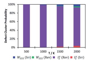
Fig. 6 Defect cluster probability as a function of temperature. The probability has been calculated relative to the most stable cluster for all concentrations. Reversible  $W_{222}$  shown in green, irreversible  $W_{222}$  in blue, reversible  $I_2^x$ purple and irreversible  $I_2^x$ in red.
