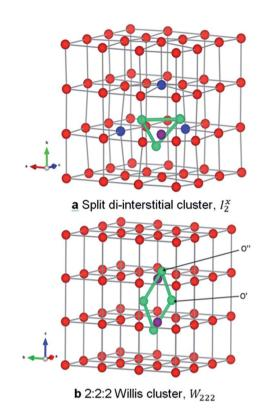
Fig. 1 Structure of oxygen defect clusters in UO<sub>2</sub>. (a) Split di-interstitial  $(I_2^X)$  and (b) 2 : 2 : 2 Willis (W<sub>222</sub>) clusters. Lattice oxygen shown in red.  $U^{4+}/U^{5+}$  are not shown for clarity. Oxygen interstitial  $(O_i'')$  shown in green. Significantly (>10%) displaced lattice oxygen shown in dark blue. Oxygen vacancies  $(V_{\circ}^{"})$  shown in purple. Bonds have been drawn in green to highlight defect cluster geometries.
