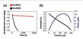
Fig. 2 (a) Normalized open circuit potential (OCP)-time curve of a 4stack PssRED (red) and normalized OCP-time curve of the NssRED (black). (b) Power (blue) and potential (black) curve of a 20-stack PssRED versus operating current.
