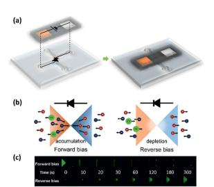
Fig. 4 (a) Equivalent circuit and schematic diagram of a polyelectrolyte ionic diode powered by a PssRED. (b) Working principle of the polyelectrolyte ionic diode system under each bias. (c) Temporal fluorescence images of the n-type polyelectrolyte gel (forward bias: upper row and reverse bias: lower row).
