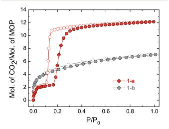
Fig. 3 CO<sub>2</sub> sorption isotherms for compounds 1-a and 1-b, measured at 195 K. Filled circles represent adsorption and empty symbols desorption in the colours indicated
