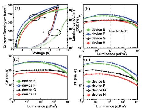
Fig. 6 (a) Current density-voltage-brightness characteristics, (b) EQE *versus* luminance curves, (c) current efficiency *versus* luminance curves, and (d) power efficiency *versus* luminance curves of the non-doped devices (E-H).
