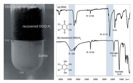
Fig. 8 Left: Recovery of DDQ-H<sub>2</sub> using celite packed fritted column (See Fig. S24 for colour image†). Right: IR spectra (cropped region) of (a) DDQ and; (b) recovered DDQ-H<sub>2</sub>. Characteristic differences in the spectra are highlighted with in blue.
