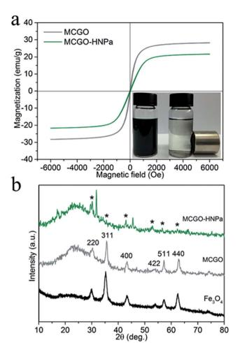
Fig. 3 (a) Magnetization loops of MCGO and MCGO-HNPa composite at 300 K. The lower right is the photo of MCGO-HNPa in aqueous solutions without and with a magnet. (b) XRD patterns of pure Fe<sub>3</sub>O<sub>4</sub>, MCGO and MCGO-HNPa, respectively.
