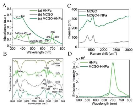
Fig. 2 (A) UV-vis spectra of (a) HNPa, (b) MCGO, (c) MCGO-HNPa; (B) FTIR spectra of CS, HNPa MCGO, MCGO-HNPa. (C) Raman spectra of nanomaterial MCGO and MCGO-HNPa composite upon laser excitation at 490 nm. (D) Fluorescence emission spectra of HNPa and MCGO-HNPa. The samples were adjusted to contain the same amount of HNPa and excited at 430 nm.
