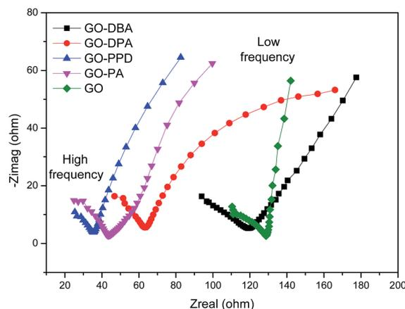
Fig. 14 Electrochemical impedance spectroscopy (EIS) of GO and the amine-functionalized electrodes in aqueous 1.0 M H<sub>2</sub>SO<sub>4</sub> electrolyte solution.
