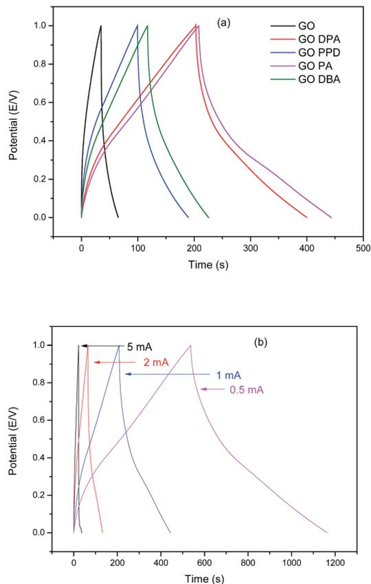
Fig. 12 Galvanostatic charge–discharge curves in 1.0 M H<sub>2</sub>SO<sub>4</sub> for (a) GO and amine-functionalized GO at 1.0 mA cm<sup>-2</sup> and for (b) GO-DPA at different current densities.
