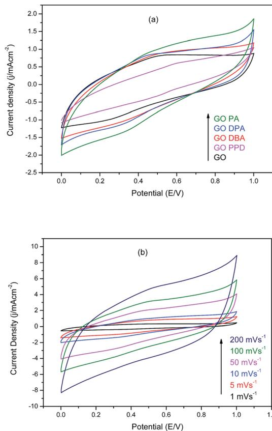
Fig. 11 Cyclic voltammograms in 1.0 M H<sub>2</sub>SO<sub>4</sub> of (a) amine-functionalized GOs at 10 mV s<sup>-1</sup> and (b) GO-PA at different scan rates.
