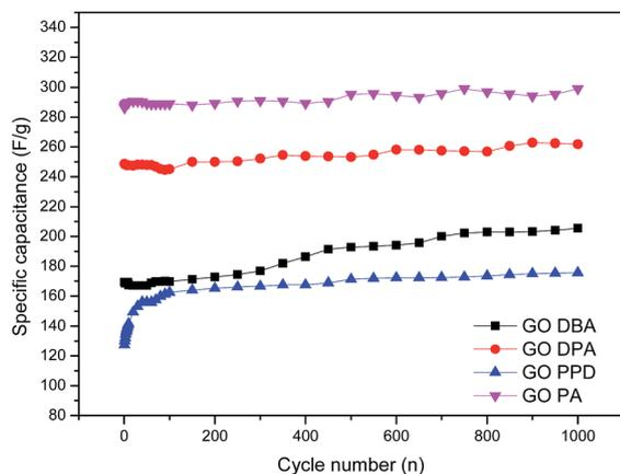
Fig. 13 Cyclic stability tests for the amine-functionalized electrodes at 1 mA cm<sup>-2</sup> discharge current density in aqueous 1.0 M H<sub>2</sub>SO<sub>4</sub> electrolyte solution.
