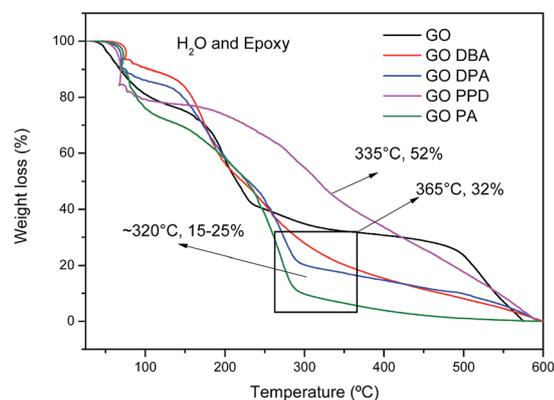
Fig. 6 TG curves of GO, GO-DBA, GO-DPA, GO-PPD and GO-PA.
