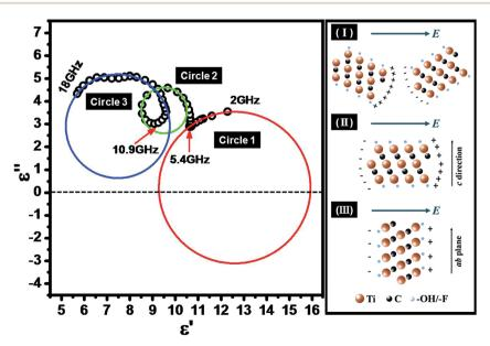
Fig. 4 Typical Cole-Cole diagram over 2-18 GHz and three typical electric polarization in Ti<sub>3</sub>C<sub>2</sub> composites.
