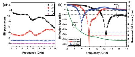
Fig. 3 (a) Dielectric and (b) microwave absorbing properties of Ti<sub>3</sub>C<sub>2</sub> nano-sheets/paraffin composites.
