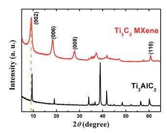
Fig. 1  $\,$  XRD patterns of pressureless-sintered  $\,$  Ti $_3$ AlC $_2$  and as-derived  $\,$  Ti $_3$ C $_2$  MXene.
