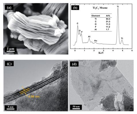
Fig. 2 (a) Cross-section SEM image of  $Ti_3C_2$  particles; (b) EDS spectrum of  $Ti_3C_2$  MXene, revealing the chemical composition of MXene; (c) cross-section TEM image of a 4-layer  $Ti_3C_2$  flake, the estimated inter-layer space is about 1 nm; (d) TEM image of a 2-layer  $Ti_3C_2$  flake.
