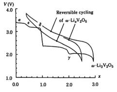
Fig. 2 Various phases associated with the electrochemical intercalation of lithium into V<sub>2</sub>O<sub>5</sub>.40
