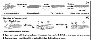
Fig. 7 (a) Schematic of possible formation process of  $V_2O_5$ -HNbs, and (b) advantages of hierarchical nanobelt structures when applied in lithium-ion batteries. <sup>82</sup>
