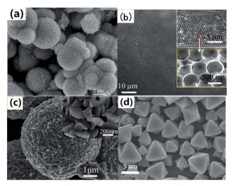
Fig. 10 (a) SEM images of  $V_2O_5$  precursor.<sup>96</sup> (b) Multilayer  $V_2O_5$  hollow sphere arrays (cross-sectional SEM images in inset).99 (c) SEM images of the V<sub>2</sub>O<sub>5</sub> product synthesized by annealing the corresponding VEG precursors in air. 101 (d) FESEM images of ammonium vanadium oxide octahedrons.102
