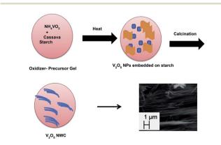
Fig. 4 Illustration of V<sub>2</sub>O<sub>5</sub> NWC formation.<sup>69</sup>
