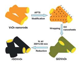
Fig. 14 Schematic of the fabrication of rGO enwrapped V<sub>2</sub>O<sub>5</sub> nanorods.140
