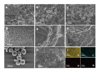
**Fig. 2** (a) and (d) Low- and high-magnification SEM images of MF-P. (b) and (e) Low- and high-magnification SEM images of NCF/CNT. (c) and (f) Low- and high-magnification SEM images of NCF/CNT/PEDOT@S. (g) High-magnification SEM image of PEDOT@S. (h) SEM image of NCF/CNT@S. (i) Corresponding elemental mapping of sulfur, carbon, oxygen, and nitrogen in the NCF/CNT/PEDOT@S electrode.
