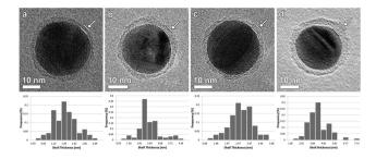
Fig. 2 BF-TEM images of (a) Aq-L4, (b) Aq-L6, (c) Aq-L8 and (d) Aq-L12 and corresponding distribution of the shell thicknesses.
