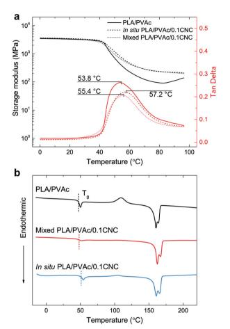
Fig. 9 (a) Dynamic mechanical analyses and (b) DSC thermograms of the PLA/PVAc, mixed PLA/PVAc/0.1CNC and *in situ* PLA/PVAc/0.1CNC.
