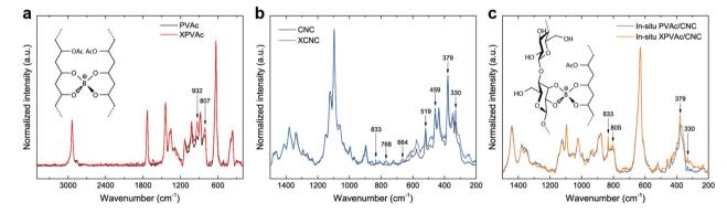
Fig. 3 (a) Raman spectra of PVAc and XPVAc films in a spectral range of 200-3500 cm<sup>-1</sup>, and the chemical structure of borax-crosslinked PVAc chains. (b) Raman spectra of CNCs and XCNCs in a spectral range of 200-1500 cm<sup>-1</sup>. (c) Raman spectra of in situ PVAc/CNC and in situ XPVAc/CNC films (weight ratio of PVAc to CNCs is 80:20), and a possible chemical structure of borax-crosslinked PVAc-CNCs.
