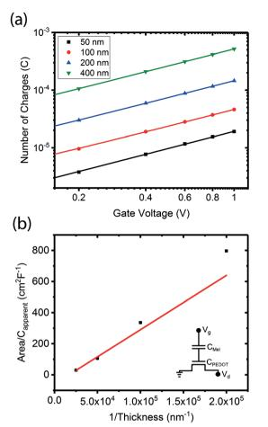
Fig. 4 Capacitance measurements. (a) Charge injected into the OECT channel as a function of  $V_q$  for different PEDOT:PSS channel thicknesses while maintaining a melanin top gate of 70 nm. (b) The inverse capacitance against inverse thickness of the PEDOT:PSS channel. Inset shows our device to be a transistor with a two capacitor gate.
