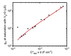
Fig. 5 Transconductance at saturation. Transconductance at saturation calculated from the measured output characteristics (at  $V_{\alpha}$  = 0 V) for multiple devices with different channel thicknesses. The red line shows a linear fit as predicted from eqn (3) and (4).
