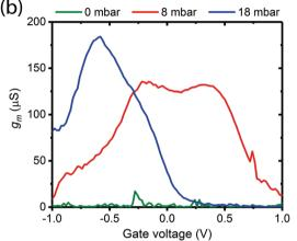
Fig. 3 (a) Hydration dependent transfer characteristics of a melanin-based OECT at 0 mbar water vapour pressure (green line), 8 mbar (red line) and 18 mbar (blue line). On/off ratio is approximately 220 at 8 mbar and approximately 10<sup>4</sup> at 18 mbar pressure. The noise at 0 mbar is negligible compared with the scale of the transfer curves. (b) The corresponding transconductance (forward sweep), which reaches 175 µS at its peak.
