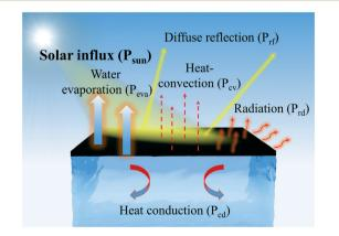
**Fig. 2** Energy balance diagram of a solar water evaporation system based on interfacial heating. Note: water evaporation is in open air in this case.
