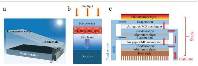
Fig. 4 (a) Simple solar distillation apparatus based on interfacial heating, (b) conceptual design of solar-thermal interfacial heating in MD, and (c) a solar distillation design with a latent heat recovery mechanism.
