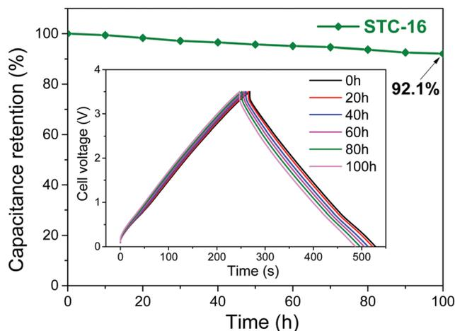
Fig. 4 Floating stability of STC-16 at a specific current of  $1 \text{ A g}^{-1}$  for 100 h of floating at 3.5 V. The inset shows the charge/discharge profiles every 20 h. Figures reproduced with permission from ref. 21.
