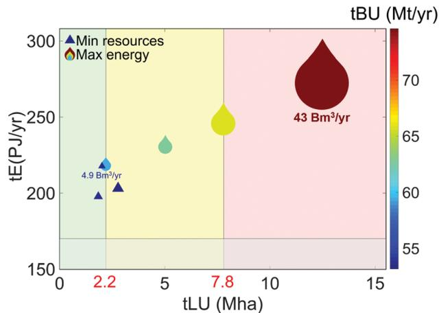
Fig. 10 BECCS total electricity generated under different land constraints, in the energy maximisation scenario (droplets), and the water, land and CO<sub>2</sub> efficiency minimisation and maximisation scenarios (triangles). Water use is represented by the colour scale, and biomass use, by the markers' size. Even when land use is constrained to a “safe” value (green zone), the UK electricity generation objective consistent with a 50 Mt<sub>CO<sub>2</sub></sub> per year target is met.
