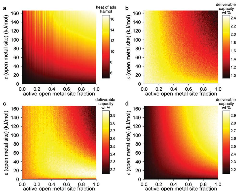
Fig. 5 Results of a GCMC study investigating the effect of active open metal site fraction and Lennard–Jones  $\epsilon$  parameter on the  $\text{H}_2$  capacity of a model system based on the  $\text{Mg}_2(\text{dobdc})$  structure type. (a) Heat of adsorption for  $\text{H}_2$  at low loading; usable capacity at (b) 77 K; (c) 180 K; and (d) 243 K given a pressure swing between 100 and 5 bar.
