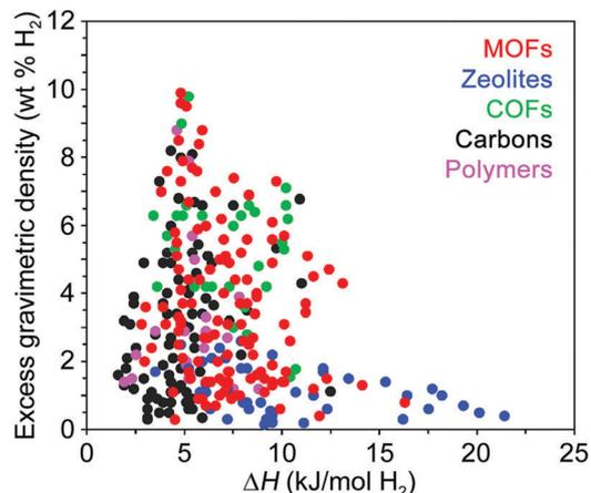
**Fig. 4** Excess gravimetric H<sub>2</sub> uptake versus enthalpy of H<sub>2</sub> adsorption for various classes of hydrogen storage materials. The adsorption enthalpy values were taken from ref. 26 and 30–33 and are reported at cryogenic conditions, typically between 77 and 87 K.
