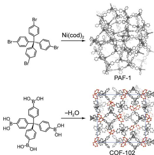
Fig. 10 Schematic representation of the synthesis of PAF-1 (top) and COF-102 (bottom).<sup>204,208</sup> Gray, red, and orange spheres represent C, O, and B atoms, respectively; quaternary carbon atoms are shown as grey tetrahedra and H atoms of the triphosphine ligands are omitted for clarity.
