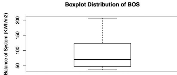
Fig. 1 Distribution in the cumulative electrical energy demand for the balance of system (CE<sub>e</sub>D<sub>BOS</sub>) on a per unit area basis [kW h<sub>e</sub> m<sup>-2</sup>] from our meta-analysis. The 0, 25, 50, 75, and 100 percentile values are, respectively, 36.58, 47.52, 70.59, 123.55, and 206.36 kW h<sub>e</sub> m<sup>-2</sup>.
