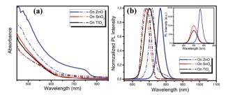
Fig. 1 (a) UV-vis absorption spectra and (b) normalized PL spectra of perovskite films deposited on different substrates before (dashed lines) and after (solid lines) vacuum-processing. The inset shows the PL spectra of the perovskite films before and after vacuum-processing.
