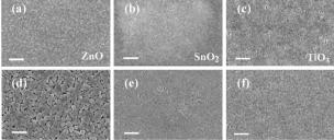
Fig. 3 SEM images of perovskite films deposited on ZnO, SnO<sub>2</sub> and TiO<sub>4</sub> substrates before (a-c) and after (d-f) vacuum-processing, respectively. The scale bar is 1 um
